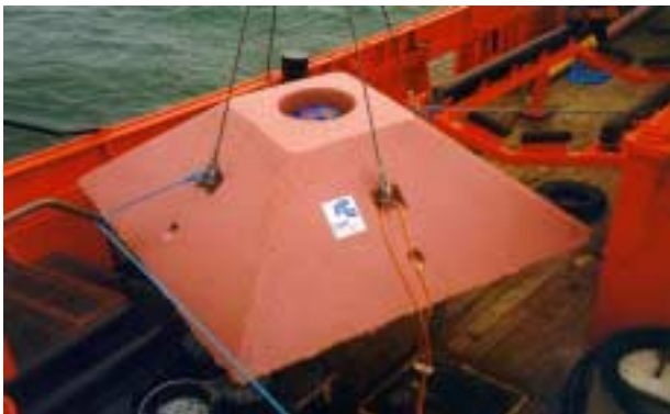
Fig. 2. ADCP installed in its mooring mount.
