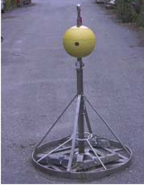
Fig. 1. S4 Current Meter in its mooring frame.
