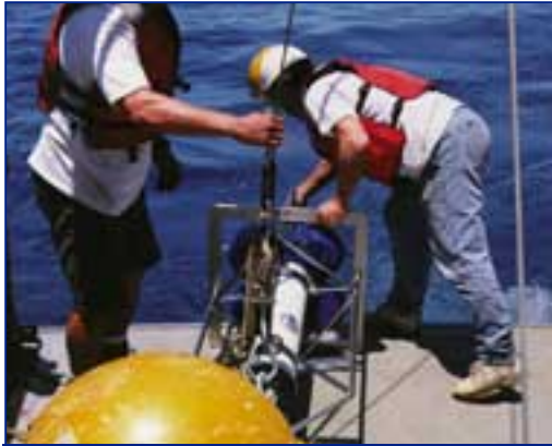
Launching a deepwater ADCP from an oceanographic research vessel.
